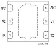
Figure 2. SKY13314-374LF Pinout (Top View)
