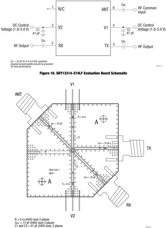
Figure 11. SKY13314-374LF Evaluation Board Assembly Diagram
