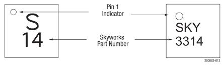
Figure 13. Typical Part Markings (Top View)
