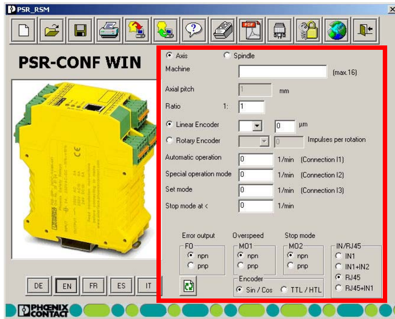
Figure 6-2 Start screen of the parameterization software
