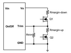
Figure 36: Circuit configuration for output voltage margining
