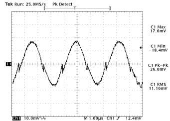
Figure 13: Output ripple & noise at 12Vin, 5V/20A out.
