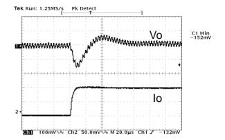
**Figure 25:** Typical transient response to step load change at  $5A/\mu S$  from 100% to 50% of lo, max at 12Vin, 5.0V out (Cout = 1uF+ 100 $\mu$ F ceramic, 470 $\mu$ F poscap).
