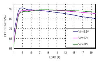
*Figure 8:* Converter efficiency vs. output current (3.3V output voltage).
