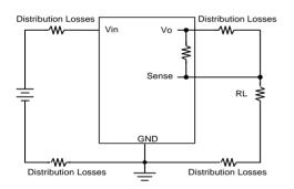
Figure 33: Effective circuit configuration for remote sense operation
