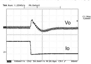
**Figure 24:** Typical transient response to step load change at  $5A/\mu S$  from 100% to 50% of lo, max at 12Vin, 5.0V out (Cout = 1uF+ 100 $\mu$ F ceramic, 470 $\mu$ F poscap).
