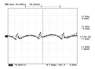
Figure 10: Output ripple & noise at 12 Vin, 0.75 V/20A out.
