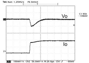
**Figure 19:** Typical transient response to step load change at  $5A/\mu S$  from 50% to 100% of lo, max at 12Vin, 0.75V out (Cout = 1uF+ 100 $\mu$ F ceramic, 470 $\mu$ F poscap).
