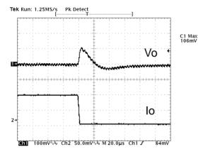
**Figure 22:** Typical transient response to step load change at  $5A/\mu S$  from 100% to 50% of lo, max at 12Vin, 2.5V out (Cout = 1uF+ 100 $\mu$ F ceramic, 470 $\mu$ F poscap).
