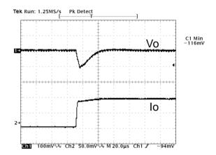
**Figure 21:** Typical transient response to step load change at  $5A/\mu S$  from 100% to 50% of lo, max at 12Vin, 1.2V out (Cout = 1uF+ 100 $\mu$ F ceramic, 470 $\mu$ F poscap).
