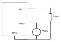
Figure 35: Circuit Configuration for programming output voltage using external voltage source
