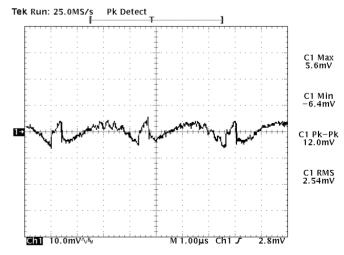
Figure 11: Output ripple & noise at 12Vin, 1.2V/20A out.
