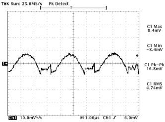
Figure 12: Output ripple & noise at 12 Vin, 2.5V/20A out.
