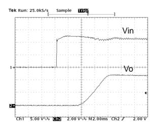
**Figure 16:** Turn on delay with external capacitors (Co= 5000  $\mu$ F), at 12vin, 5.0V/20A out. DS\_DNL10SIP20\_01302015
