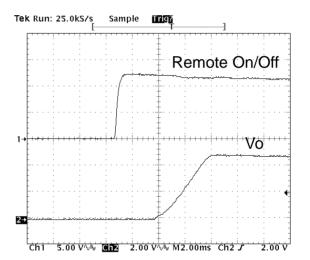
*Figure 15:* Turn on delay time using Remote On/Off, at 12vin, 5.0V/20A out.
