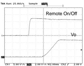
**Figure 17:** Turn on Using Remote On/Off with external capacitors (Co=  $5000 \ \mu$ F),  $5.0V/20A \ out$ .
