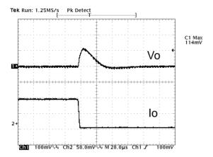
**Figure 20:** Typical transient response to step load change at  $5A/\mu S$  from 100% to 50% of lo, max at 12Vin, 1.2V out (Cout = 1uF+ 100 $\mu$ F ceramic, 470 $\mu$ F poscap).
