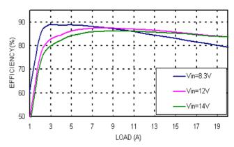
*Figure 2:* Converter efficiency vs. output current (1.0V output voltage).
