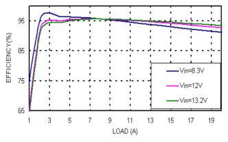
*Figure 9:* Converter efficiency vs. output current (5.0V output voltage).
