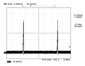
*Figure 26:* Output short circuit current 12Vin, 0.75Vout (10A/div).
