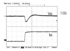
**Figure 23:** Typical transient response to step load change at  $5A/\mu S$  from 50% to 100% of lo, max at 12Vin, 2.5V out (Cout = 1uF+ 100 $\mu$ F ceramic, 470 $\mu$ F poscap).
