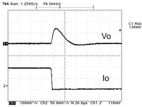
**Figure 18:** Typical transient response to step load change at  $5A/\mu S$  from 100% to 50% of lo, max at 12Vin, 0.75V out (Cout = 1 $\mu$ F + 100 $\mu$ F ceramic, 470 $\mu$ F poscap).
