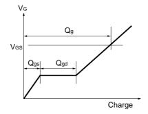
Fig.13 Gate Charge Waveform
