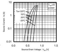
Fig.6 Source-Current vs. Source-Drain Voltage
