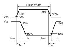
Fig.11 Switching Time Waveforms
