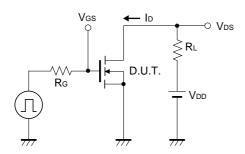
Fig.10 Switching Time Test Circuit
