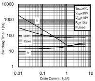
Fig.8 Switching Characteristics
