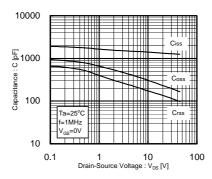
Fig.7 Typical capacitance vs. Source-Drain Voltage
