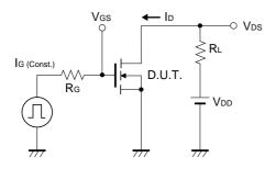
Fig.12 Gate Charge Test Circuit
