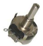
53 Series Industrial Potentiometer, Conductive Plastic Element, Solder lug Terminals, 2 W Power Rating, 15 kOhm Resistance Value
