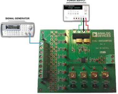
Figure 1. EVAL-ADG5208FEBZ, Power Supply, and Signal Generator
