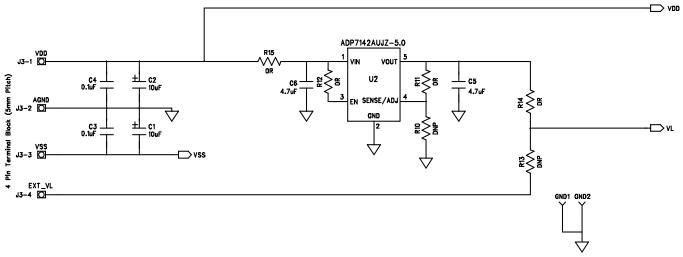
Figure 5. ADG5208F Evaluation Board Schematic (Part 3)
