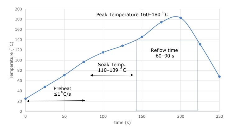
**The Preheat Zone**, which is also referred to as the ramp zone, is used to elevate the temperature of the PCB to the desired soak temperature. In the preheat zone, the rate of temperature rise should not exceed 2.5 °C/s to avoid thermal chock stresses. The oven preheat zone normally occupies 25–33% of the heated tunnel length.
