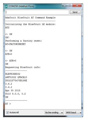
To send an AT command to the Bluefruit LE module, enter the command in the textbox at the top of the Serial Monitor and click th**Send** button:
