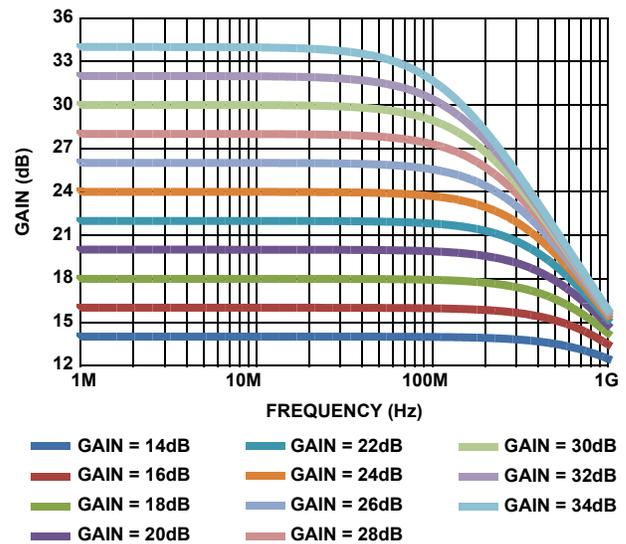
FIGURE 11. PARAMETRIC RESPONSE CURVES FOR 75Ω INPUT DESIGNS
