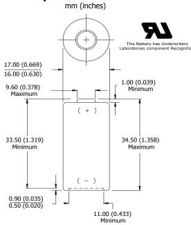
This battery contains a Positive Temperature Coefficient (PTC) safety device to limit current during short circuit conditions.
