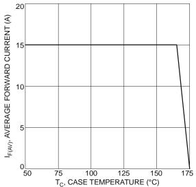
Fig. 3 Forward Current Derating Curve, Per Element
