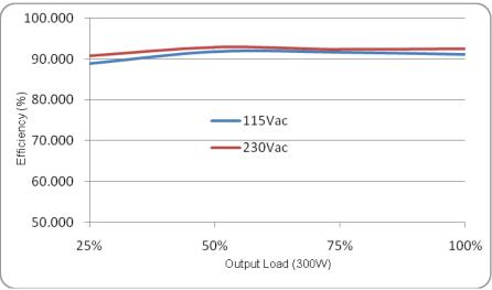
Fig.1 Efficiency versus output load
