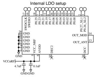
Internal LDO setup with external 32.768kHz X'tal
