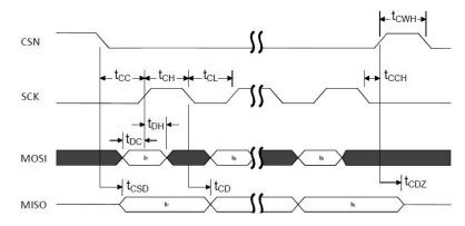
SPIS timing diagram, one byte transmission, SPI Mode 0
