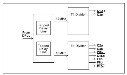
Figure 5 - Output Interface Circuit Block Diagram
