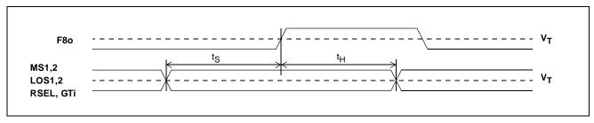
Figure 21 - Input Controls Setup and Hold Timing
