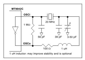
Figure 10 - Crystal Oscillator Circuit
