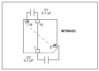
Figure 17 - Power Supply Decoupling
