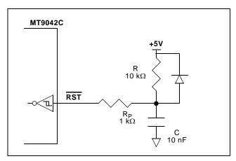
Figure 15 - Power-Up Reset Circuit
