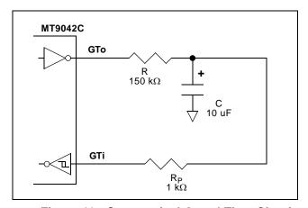
Figure 11 - Symmetrical Guard Time Circuit
