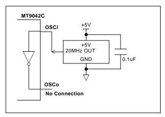
Figure 9 - Clock Oscillator Circuit
