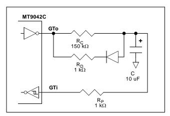
Figure 13 - Unsymmetrical Guard Time Circuit
