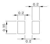
Mask open area ratio:80% Mask thickness:80~100um
