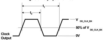
Figure 9. Rise Time =  $T_{RF}$ , Fall Time =  $T_{RF}$
