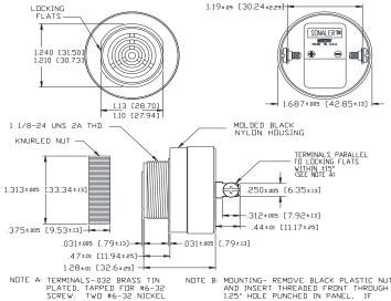
NOTE A: TERMINALS-032 BRASS TIN PLATED, TAPPED FOR #6-32 SCREW. TWD #6-32 NICKEL PLATED BRASS SCREWS INCLUDED. WILL ACCEPT 1/4\* QUICK CONNECT.
