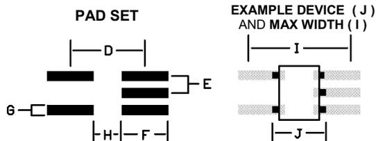
MOUNTING PADS ARE OVERSIZED IN LENGTH TO ACCEPT A WIDER RANGE OF DEVICE WIDTHS AND TOLERANCES AND TO PERMIT HAND SOLDERING.
