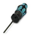
Torque screw driver with preset torque of 0.8 Nm, with 4 mm hexagon for accommodating SAC bits, two-component handle with non-slip grip
