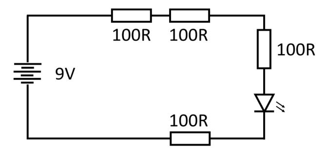
The circuit diagram for the Learn to Solder PCB is shown above. It is a very simple circuit. The 9V battery that powers the circuit is connected via the PCB pads.
