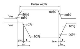
Fig.17 Switching time waveforms
