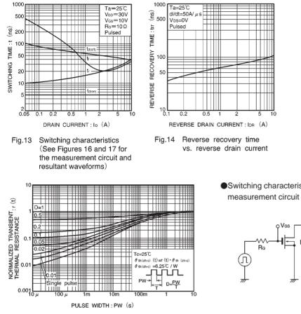
Fig.15 Normalized transient thermal resistance vs. pulse width
