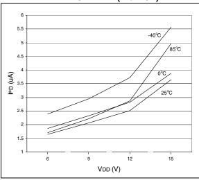
FIGURE 11-7: TYPICAL IPD vs. VDD,
