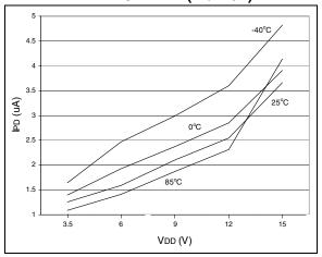
FIGURE 11-11: TYPICAL IPD vs. VDD,
