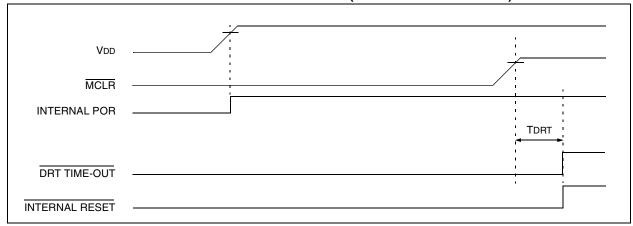
FIGURE 7-9: TIME-OUT SEQUENCE ON POWER-UP (MCLR TIED TO VDD): FAST VDD RISE TIME
