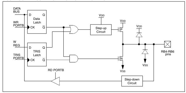
FIGURE 5-4: BLOCK DIAGRAM OF PORTB<7> PIN
