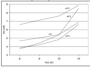
FIGURE 11-9: TYPICAL IPD vs. VDD, WATCHDOG TIMER DISABLED (Vio = 3V)
