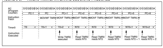
FIGURE 6-4: TIMERO TIMING: INTERNAL CLOCK/PRESCALE 1:2
