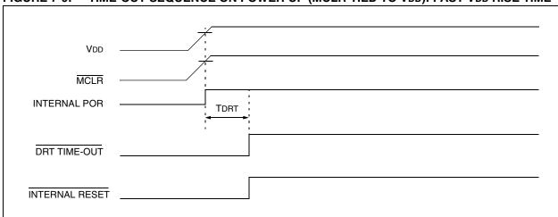
FIGURE 7-10: TIME-OUT SEQUENCE ON POWER-UP (MCLR TIED TO VDD): SLOW VDD RISE TIME
