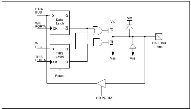
FIGURE 5-2: BLOCK DIAGRAM OF PORTB<0:3> PINS
