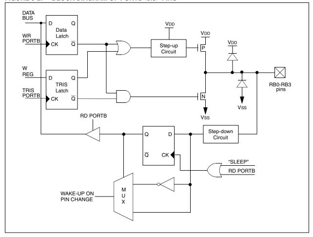
FIGURE 5-3: BLOCK DIAGRAM OF PORTB<4:6> PINS
