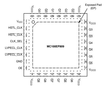
Figure 2. 32-Lead QFN Pinout (Top View)
