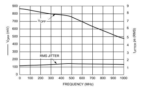
Figure 4. Output Frequency (F<sub>OUT</sub>) versus Output Voltage (V<sub>OPP</sub>) and Random Clock Jitter (t<sub>JITTER</sub>)
