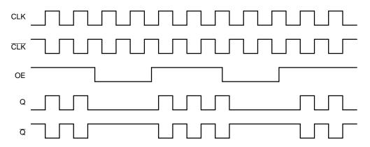
Figure 9. Output Enable (OE) Timing Diagram
