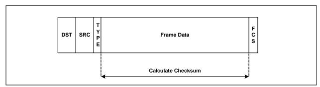
In mode 1, the RXCOE supports VLAN tags and a SNAP header. In this mode the RXCOE calculates the checksum at the start of L3 packet. The VLAN1 tag register is used by the RXCOE to indicate what protocol type is to be used to indicate the existence of a VLAN tag. This value is typically 8100h.
