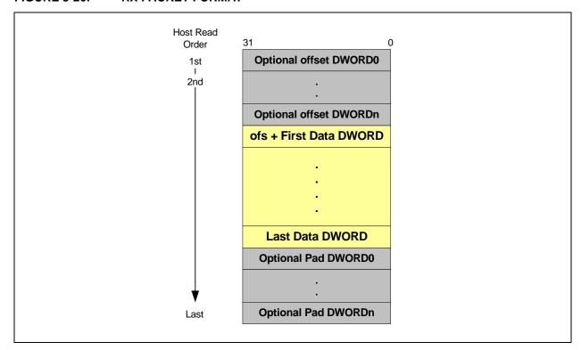
Figure 3-27 shows the RX packet format when the RX checksum is enabled. The RX checksum data appended to the data payload is treated just as an additional 4-bytes within the RX Data FIFO. The RX checksum is enabled by setting the RXCOE\_EN bit in the COE\_CR—Checksum Offload Engine Control Register. For more information on the RX checksum, refer to Section 3.6.1, "Receive Checksum Offload Engine (RXCOE)".
