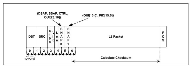
FIGURE 3-6: ETHERNET FRAME WITH VLAN TAG AND SNAP HEADER
