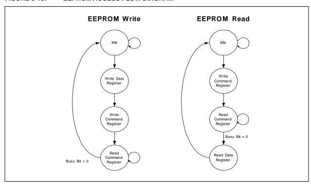
**FIGURE 3-10: EEPROM ACCESS FLOW DIAGRAM**
