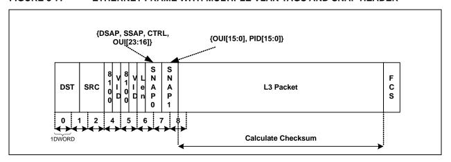
The RXCOE supports a maximum of two VLAN tags. If there are more than two VLAN tags, the VLAN protocol identifier for the third tag is treated as an Ethernet type field. The checksum calculation will begin immediately after the type field.
