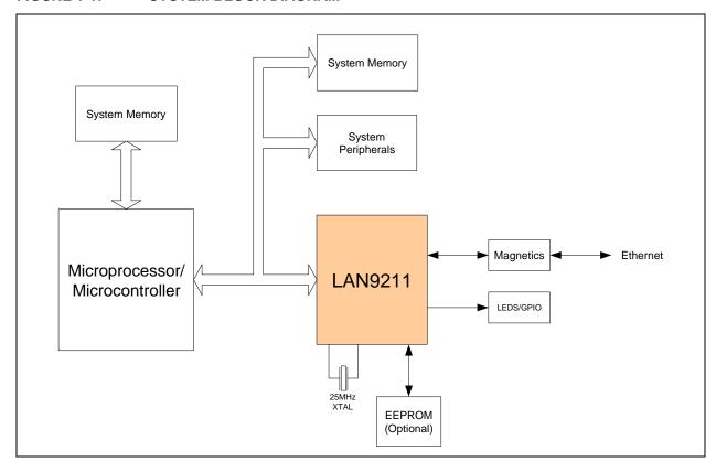
The Microchip LAN9211 integrated 10/100 MAC/PHY controller is a peripheral chip that performs the function of translating parallel data from a host controller into Ethernet packets. The LAN9211 Ethernet MAC/PHY controller is designed and optimized to function in an embedded environment. All communication is performed with programmed I/O transactions using the simple SRAM-like host interface bus.
