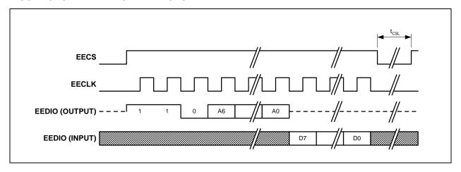
**WRITE (Write Location):** If erase/write operations are enabled in the EEPROM, this command will cause the contents of the E2P\_DATA register to be written to the EEPROM location selected by the EPC Address field (EPC\_ADDR). The EPC\_TO bit is set if the EEPROM does not respond within 30ms.
