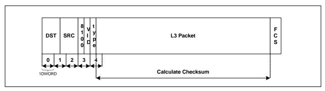
FIGURE 3-5: ETHERNET FRAME WITH LENGTH FIELD AND SNAP HEADER
