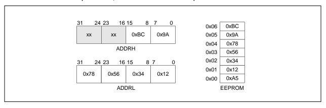
**Note:** By convention, the left most byte of the Ethernet address (in this example 0x12) is the most significant byte and is transmitted/received first.
