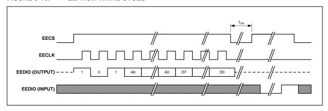
**WRAL (Write All):** If erase/write operations are enabled in the EEPROM, this command will cause the contents of the E2P\_DATA register to be written to every EEPROM memory location. The EPC\_TO bit is set if the EEPROM does not respond within 30ms.
