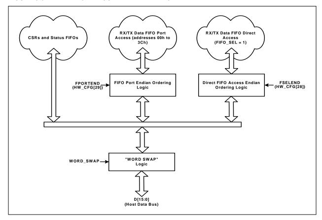
FIGURE 3-8: LAN9211 HOST DATA PATH DIAGRAM
