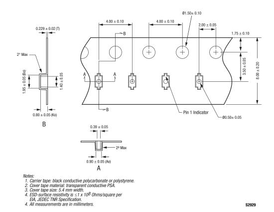
Figure 6. SC-79 Tape and Reel Dimensions
