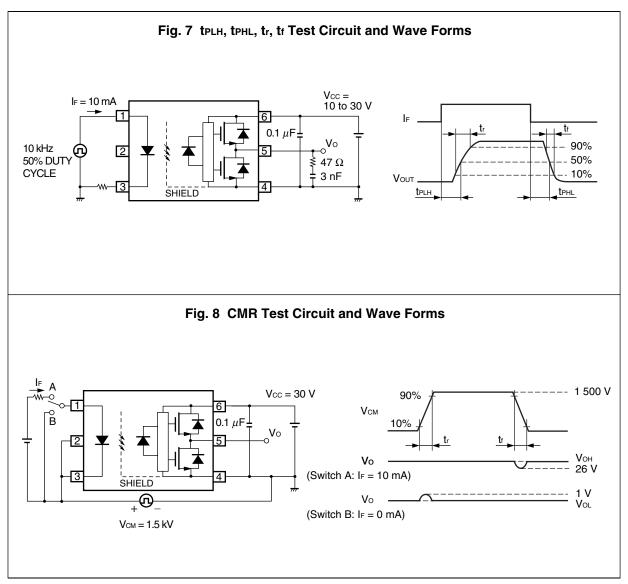
**Remarks 1.** Common Mode Transient Immunity at High Level Output is the maximum value of  $dV_{CM}/dt$  at which the output remains High Level (e.g.  $V_O > 15 \text{ V}$ ).
