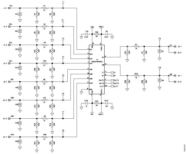
Figure 3. ADG5249F Evaluation Board Schematic (Part 1)
