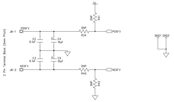
Figure 5. ADG5249F Evaluation Board Schematic (Part 3)
